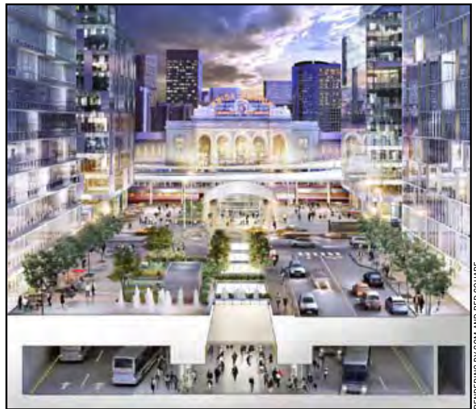
Bus facility beneath street and linear park at Denver Union Station.
